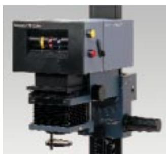
The height can be adjusted quickly to millimetre accuracy by a handgrip with quick-release coupling. A counterweight spring balances the weight. The column is marked with centimetre and inch scales as well as magnification factors for rapidly resetting a particular print size.
