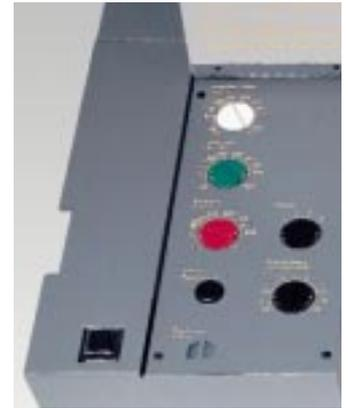
The **replenishment module** is equipped with efficient bellows pumps. A sensor bar integrated in the paper feed section scans the amount of material passing across it and carries out a replenishment cycle for each 0.1 m<sup>2</sup> of material. The individual replenishment rates for each bath are set via colour-coded rotary potentiometers. An LED display signals which processing track is occupied and goes off as soon as the sheet has been completely fed in.
