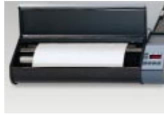
The **exposed photographic paper** is fed into the first bath via a guide plate and feed rollers. Large prints can be fed into the lower part of the feed section so that the flap can be closed as soon as the sheet has been inserted. A precisely controlled drive motor and large pairs of rollers guarantee smooth paper transport.
