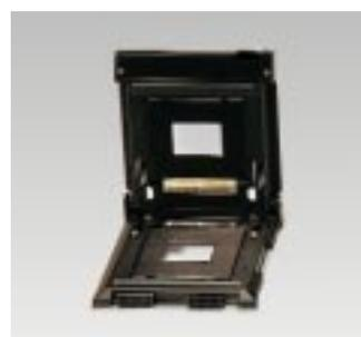
The professional film carrier is made of diecast aluminium, and features adjustable masking strips, register pins and automatic centering. With the aid of interchangeable metal masks and glass plates, the film carrier can be used for formats up to 6 x 7 cm (2<sup>1</sup>/<sub>4</sub> x 2<sup>1</sup>/<sub>4</sub> in) and APS.
