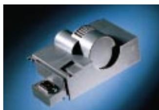
Energy Mot drives the tank's rollers and spiral agitator.
