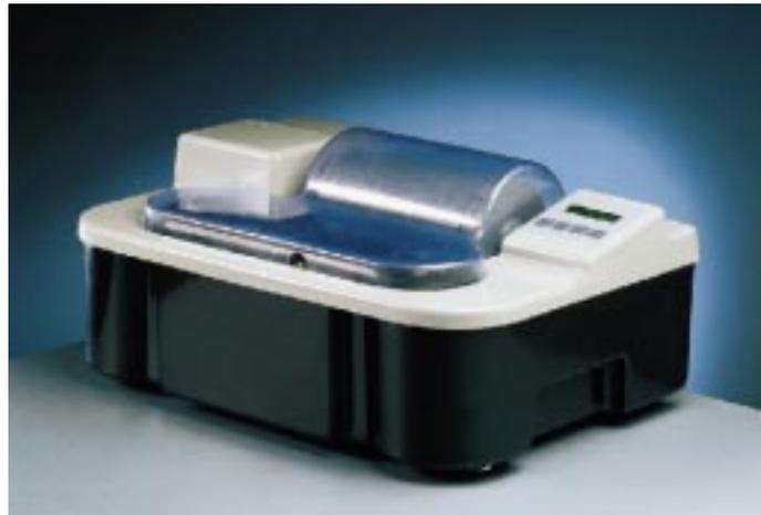
As soon as the process temperature has been reached, the first chemical is pumped into the tank. Then, after the required time has elapsed, it is emptied and collected. The rinse water, adjusted automatically to the right temperature, is pumped in from the water jacket. The current bath temperatures are continuously displayed on an LCD (in °C or °F). A total of ten different processes can be freely programmed, with the most important of them having been preset in the factory (E6, C41, B/W).
