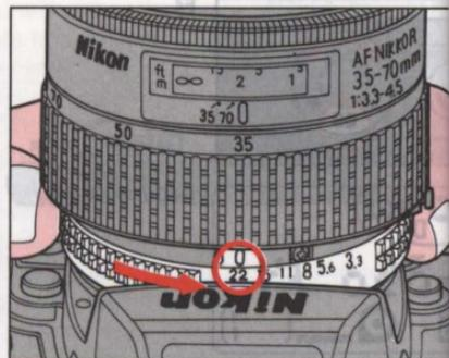
2. Set lens to minimum aperture (i.e., highest f-number). If not properly set, the shutter locks. (F4 shutter displays FEE, but will fire.)
