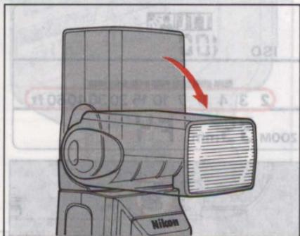
9. Tilt the flash head to normal shooting position, and confirm flash head is locked.
