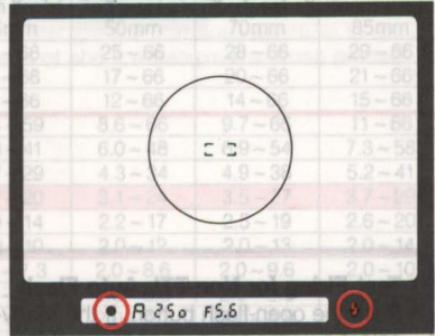
**5.** Lightly press the shutter release button and confirm the ready-light and in-focus indicator have come on.
