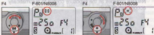
To select either Matrix Metering or Center-Weighted Metering, use the F-801/N8008's metering system selection button, or for the F4, selection dial.
