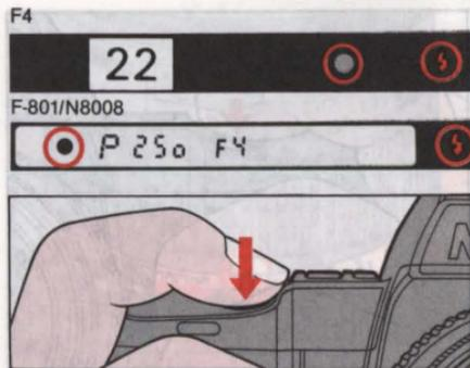
4. Confirm the ready-light and in-focus indicator are on, then fully depress the shutter release button to take the picture.
