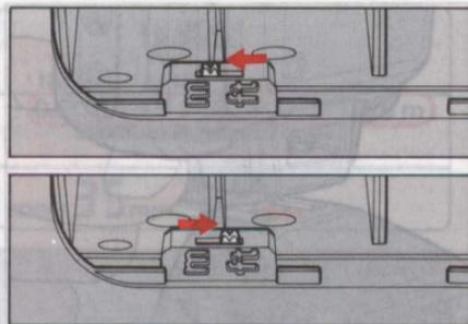
2. Slide the meter/feet lever to select the desired indication (meters or feet) on the LCD panel. (Set at meters when shipped from factory.)
