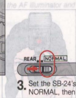
**3.** Set the SB-24's flash mode selector to TTL and the flash sync mode selector to NORMAL, then turn on the SB-24 and take the picture.
