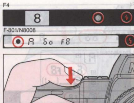
4. Confirm the ready-light and in-focus indicator are on, then fully depress shutter release button to take the picture.
