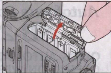
Slide the battery chamber cover in the direction of the ▼ and lift to open.
