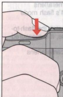
3. Confirm the in-focus indicator lights up, then fully depress the shutter release button.
