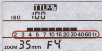
The shooting distance scale in the LCD panel can be set to either meters or feet.
