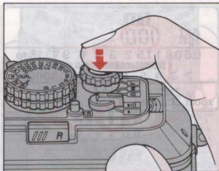
4. Lightly press the shutter release button and confirm the ready-light and in-focus indicator are on.
