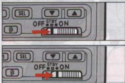
Set the power switch to STBY (standby position) or ON to turn on the SB-24.
