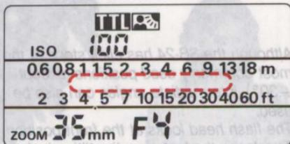
When the flash head is tilted up or rotated away from the original position, the shooting distance indicators in the LCD panel disappear, because distance cannot be correctly calculated.
