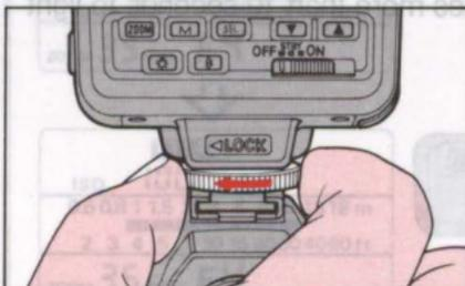
Turn locking wheel to tighten.
