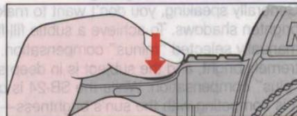
4. Confirm the ready-light and in-focus indicator are on, then fully depress shutter release button to take the picture.
