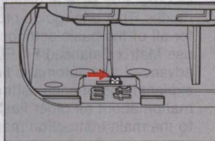
Slide the meter/feet lever to select the desired indication (meters or feet) in the LCD panel. (Originally set to meters at factory.)
