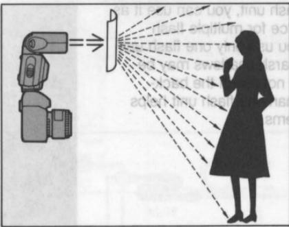
To diffuse light, place a translucent material, such as one or more sheets of tracing paper between the flash and the subject. For optimum results, experiment with different flash-to-diffuser distances and more than one diffuser. When using a diffuser, use the SB-24 in either TTL auto or manual flash mode.
