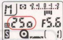
2. Set your desired shutter speed within the sync range and set your desired aperture on the lens.
