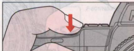
5. Confirm the ready-light and in-focus indicator are on, then fully depress shutter release button to take the picture.
