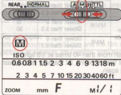
Set the SB-24's flash mode selector to M and the flash sync mode selector to your choice of NORMAL or REAR, then turn on the SB-24.
