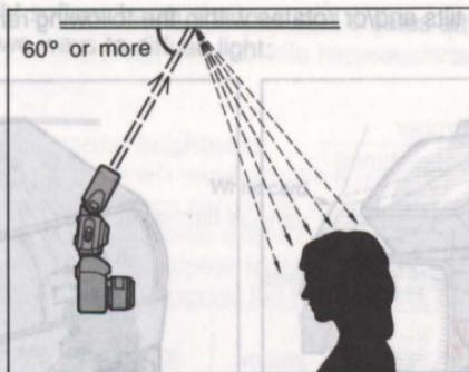
1. Select a ceiling or wall to bounce the flash from. In color photography, only use bounce with white surfaces. Otherwise, color photographs will come out with an unnatural color cast similar to that of the reflecting surface.
