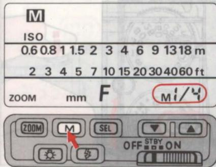
3. Press the "M" button to control the amount of light. The light output changes as follows, and is shown in the LCD panel.
