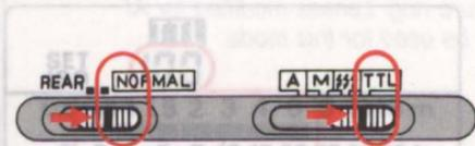
1. Set SB-24's flash mode selector to TTL, and the flash mode selector NORMAL.
