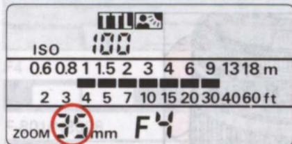
In auto mode, the zoom head automatically adjusts to provide an angle of coverage that matches the focal length of the lens in use (indicated in the LCD panel).
