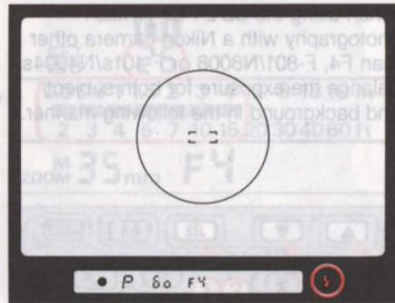
2. Lightly press the camera shutter release button and confirm that the viewfinder ready-light comes on.
