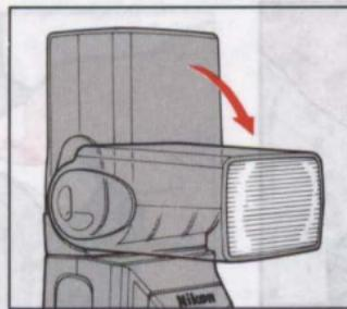
Tilt the flash head to the normal shooting position, and confirm flash head is locked.
