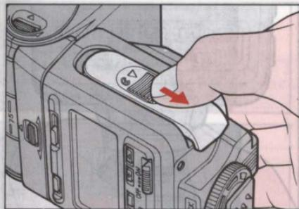
1. Slide the battery chamber cover in the direction of the ▼ and lift to open.
