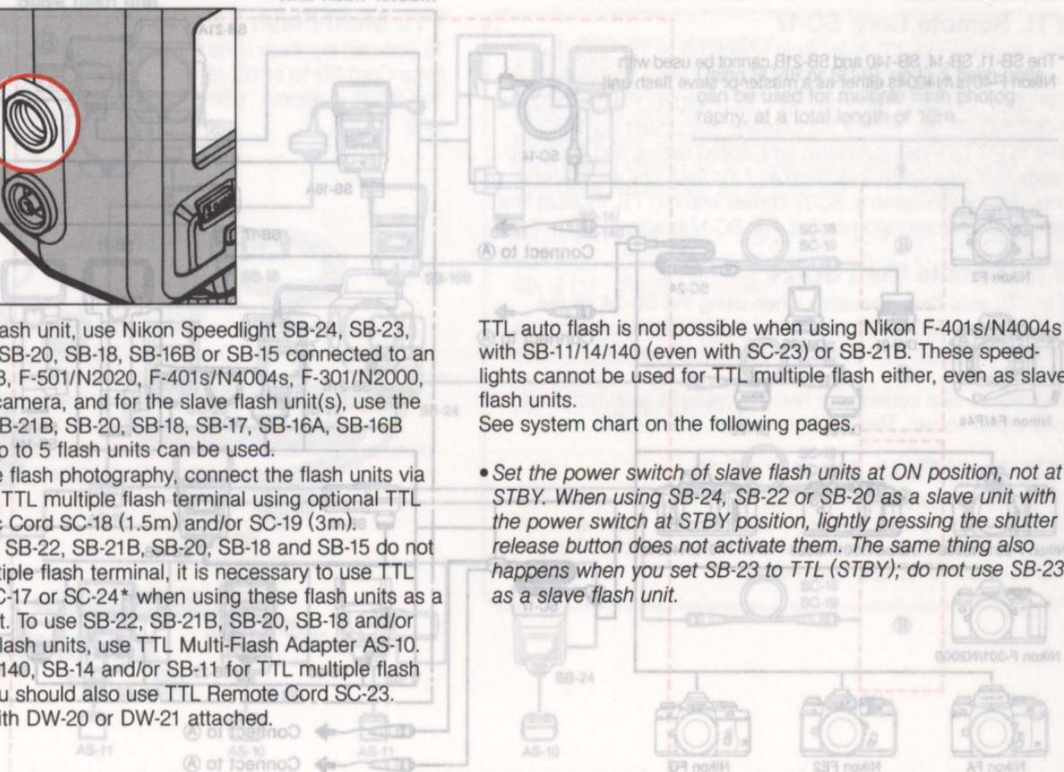
\*The SB-11, SB-14, SB-140 and SB-18 cannot be used with Nikon F-401s/N4004s either as a master or slave flash unit. This is because the TTL Multi-Flash Adapter AS-10 cannot be used for photography at a total length of 1.5m.
