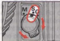
1. Set the Nikon F4, F-801/N8008 or F-501/N2020 focus mode selector to S for Single Servo Autofocus mode, or set the F-401s/N4004s to A for autofocus mode.
